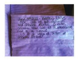
Documentation of a third party visit in June 2022, which measured a 1.5 foot deep layer of sludge in the chlorine contact basin. The operator added chlorine to the chlorinator at that time.
